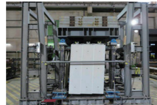
ALC外壁付き骨組の振動台実験 Shaking table test on framework with ALC exterior walls
