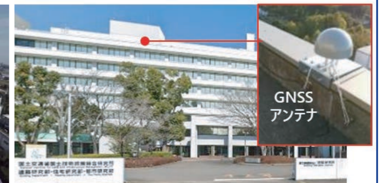
衛星技術強震観測による被害状態取得・判定支援システムの開発 Development of a Support System for Obtaining and Judging the State of Damage by Satellite Technology Strong-motion Earthquake Observation
