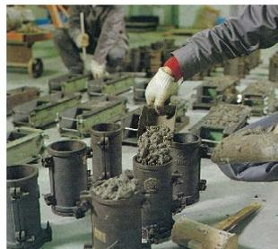
Schematic concrete specimens making
