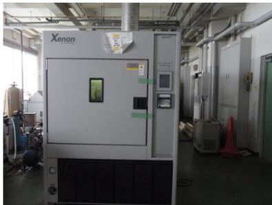
Ultraviolet accelerator facility
