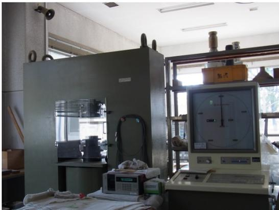
500t strength test machine with high rigidity
