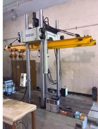
Dynamic loading-deformation testing machine
