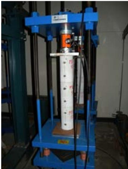
Creep Compression Test of Cylindrical
