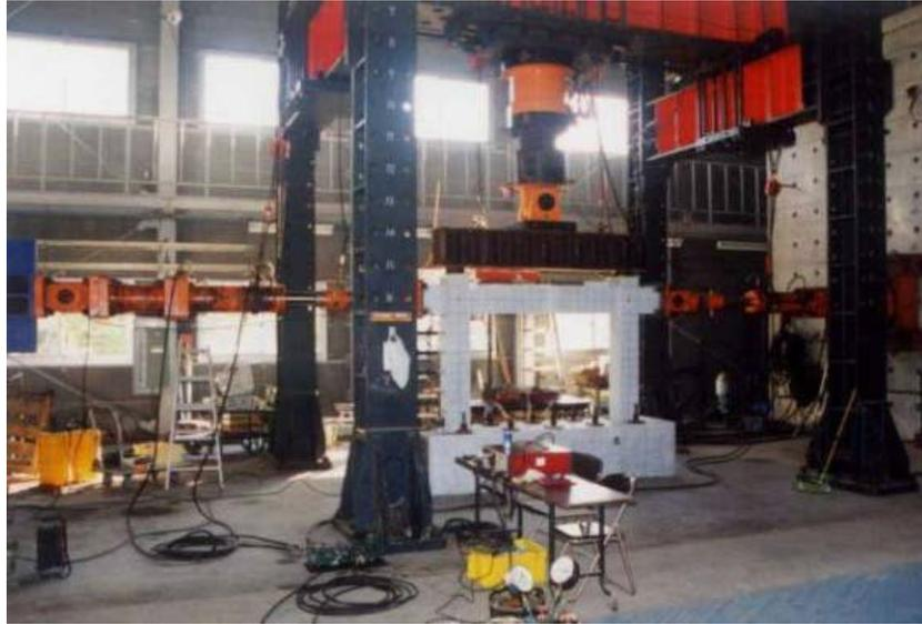
**④ 20MN Vertical and Multi Horizontal Direction Loading Test Machine**
