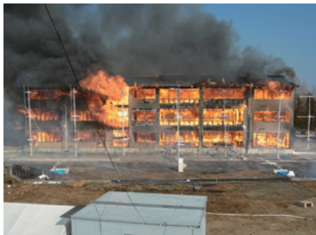
Photo 8: Three stories burning simultaneously (33 minutes after ignition)
