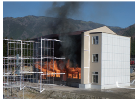
Photo 10: Flames also emerge from second floor opening (131 minutes after ignition)
