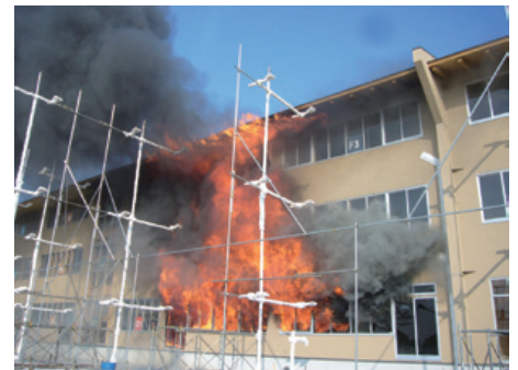
Photo 7: Fire spreading to upper floors due to emerging flames (six minutes after ignition)
