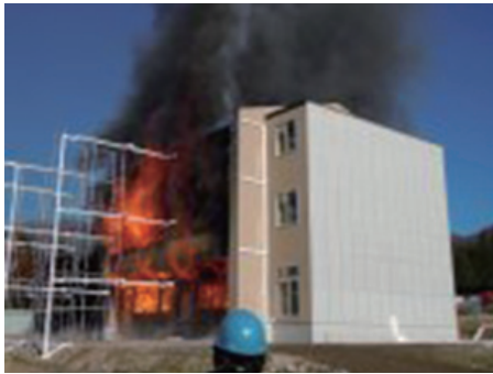
Photo 13: Fire spreads to the third floor
