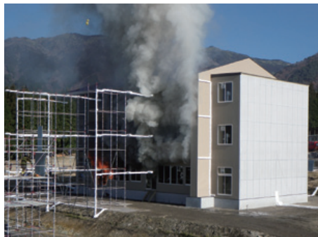
Photo 9: Flashover occurs in ignition room (89 minutes after ignition)
