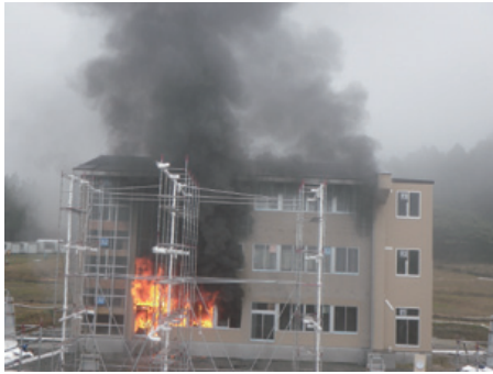
Photo 11: Flashover occurs in ignition room (68 minutes after ignition)
