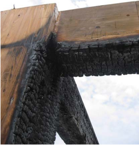
Photo 4: Fire performance after testing
