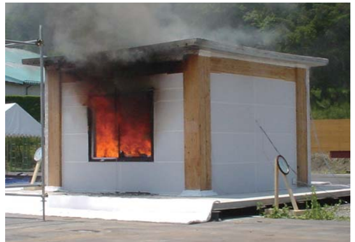
Photo 3: Full-size fire testing of a wooden hybrid construction
