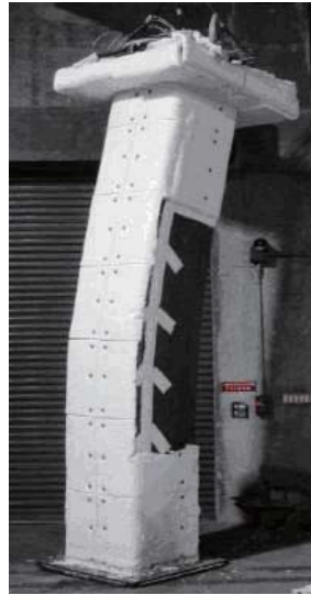
Photo 2: Test column after fire testing where 25% of the fire resistive covering was stripped off
