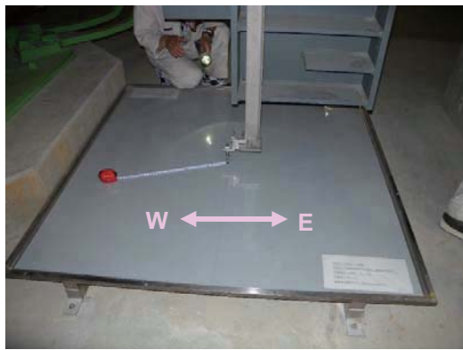
Photo 9.2-23 Trace of displacement of the SI floor on the scratch board
