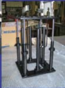
Application of the isolator to the showcase of Fukuoka City Museum (horizontal and vertical isolation)
