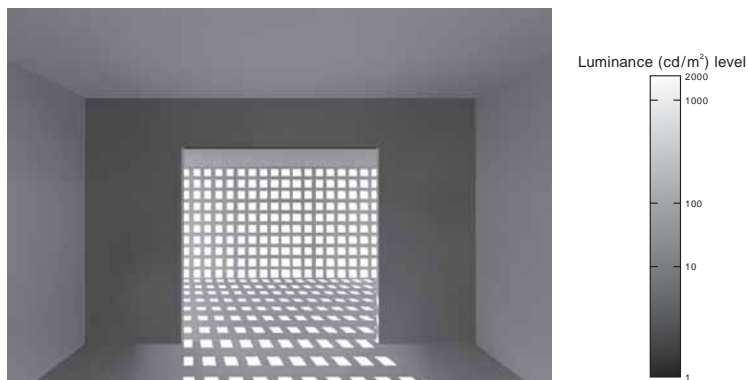
Fig. b Indoor light condition with blocks with decorative openings (luminance distribution) Luminance (cd/m 2 ) level
