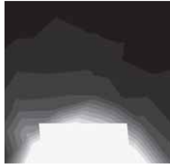
Fig. a Floor illuminance distribution with narrow space between buildings (3 m)
